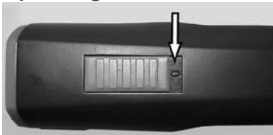
Fig. 4 Switch in OFF-position ("0")
