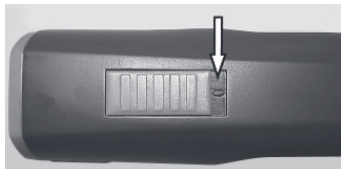
Fig. 4 Switch in OFF-position ("0")
